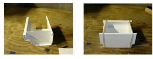
6. While the glue sets for the side pieces, cut the filter block to size or make your under gravel plate. The filter block should be approximately 2 inches long and roughly 1 inch wide. Cut a central slit in the filter block and widen the hole with a piece of tubing to the width of the pick up tube. If making the under gravel plate, complete the following steps:
