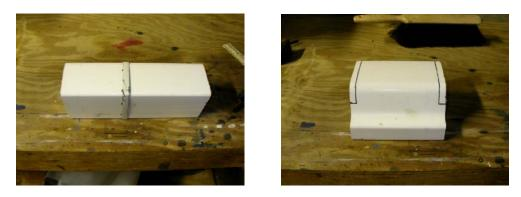
3. Using the snips or heavy duty scissors, cut along the line for the depth and cut out notches along the inside dimension of the filter. The notches will help in using the jigsaw to cut the inside dimension. Cut the inside dimension of the filter. After completing the inside dimension cut, do a quick check of the fit inside your tank. The fit should have a little play, not more than 1/8" or so.
