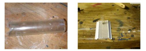
7. Also, while the glue sets, measure and cut the following pieces - the inner bottom plate and the water diffuser. The bottom plate can fit loosely inside the bottom of the filter, but the diffuser must fit snugly against the two side pieces.
