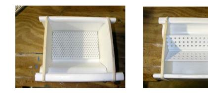
8. Once the inside pieces are cut and the glue has set, mark and drill the holes in the bottom of the filter. Also, mark and punch/drill the holes in the bottom plate and the diffuser. Be careful that the holes for the bottom plate and diffuser match up as closely as possible with the hole in the filter bottom so there is as little gap as possible.
