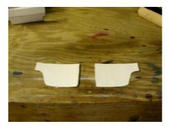
5. Insert the side pieces into the "tracks". Using rubber bands, clamp the side pieces in position as shown below. When rubber bands are in place, glue the side pieces in place on the outside of the filter body. The PVC cement will penetrate the joint sufficiently enough to seal it.
